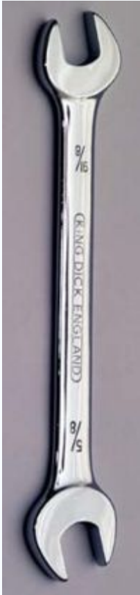
Fig. Double open-end wrench or open-ended spanner
