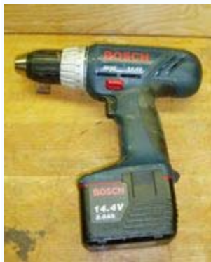
Fig. A cordless drill with clutch
