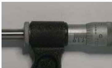
Fig. Micrometer thimble showing 0.276 inch
