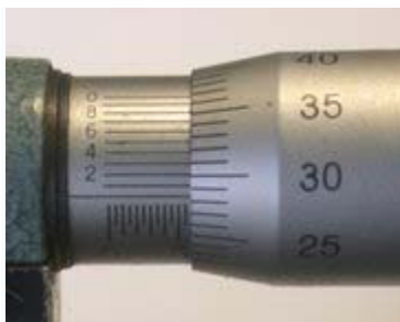
Fig. Micrometer sleeve (with vernier) reading 5.783mm
