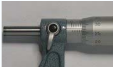
Fig. Micrometer thimble reading 5.78mm
