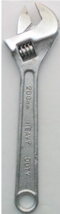
Fig. Adjustable wrench or adjustable spanner
